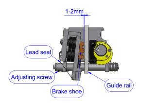
The safety gear ↓ may only be installed if the values indicated on the type plate correspond to the lift data. Check that the lead sealing is undamaged. Attach brake shoe to the rail using the adjusting screw with a gap between 1 and 2 mm.
