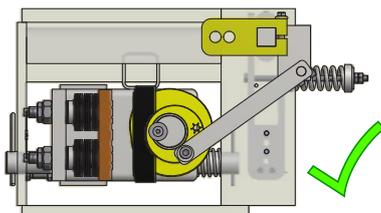
Attention: Reversing lever points outwards. Safety gear out of function!
